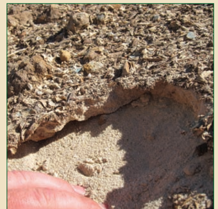
Penetrates and binds soil surface
